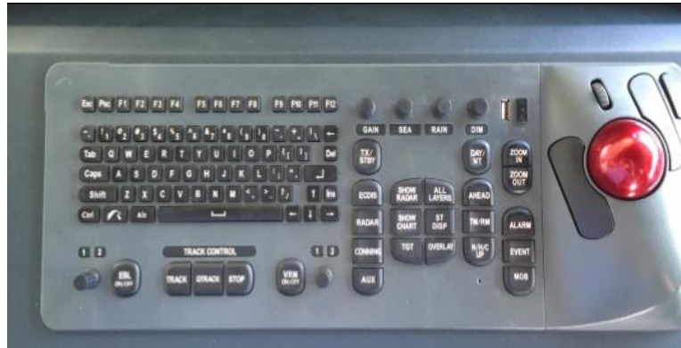
Figure 1: ECDIS keyboard with an unprotected USB input
